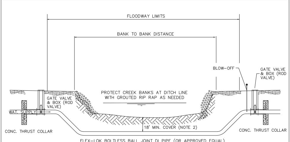
FLEX-LOK BOLTLESS BALL JOINT DI PIPE (OR APPROVED EQUAL) BACKFILL DITCH IN CREEK BED WITH FLOWABLE FILL
